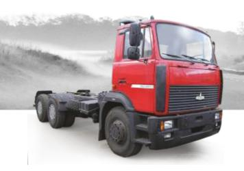
Designed for installation auto-concrete-pumps, auto-vans, truck for water, fuel transportation, washing equipments
